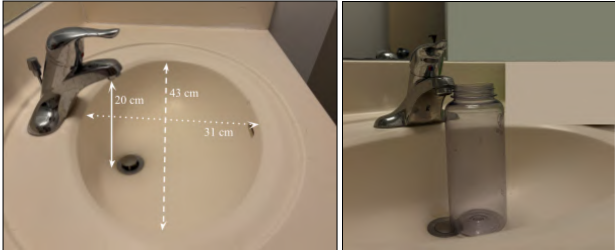
Figure 1: Dimensions of sink and tap configuration (left) and height comparison of faucet and water bottle (right).
